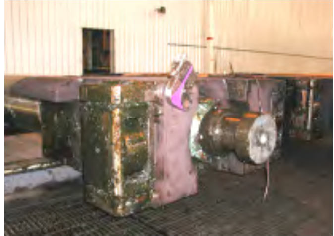
Hot Mill- Roller Cylinders Stealth-4 w 36mm Allen adaptors Torque-670 Ft Lbs- 100%
