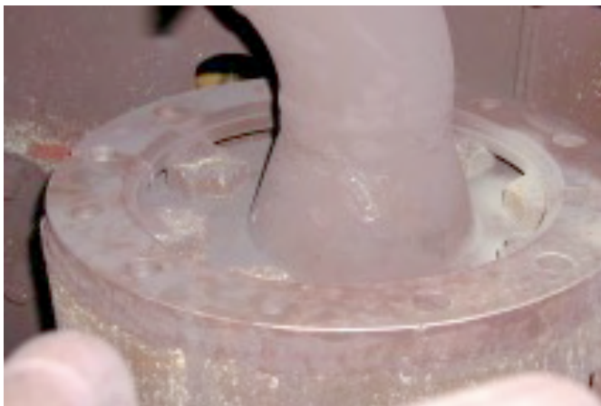
Rough Mill- Descaler Flanges Stealth-4 w 55mm link Torque 1800 Ft Lbs Torqued Pattern- 100%
