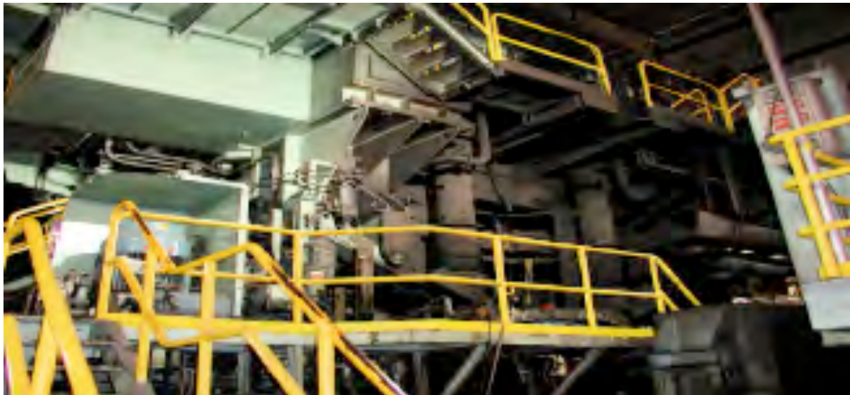
Rough Mill- Descaler Flanges Stealth-4 w 55mm link Torque 1800 Ft Lbs Torqued Pattern- 100%
